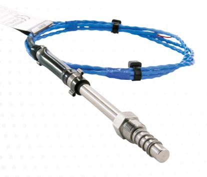
Operating on a simple reed switch and magnet technology, the Flo-Tel sensor fits into a holder with a magnet on the rupture disc. When the disc bursts, the magnet arcs away from the sensor, giving an open circuit signal.
